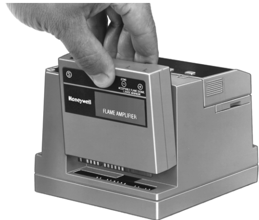
Fig. 2. Installing flame signal amplifier.
