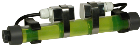
The speed of sound travelling between the two transducers varies with liquid velocity. A time-differential relationship conversion to flow rate is based on the velocity as well as the pipe diameter.
