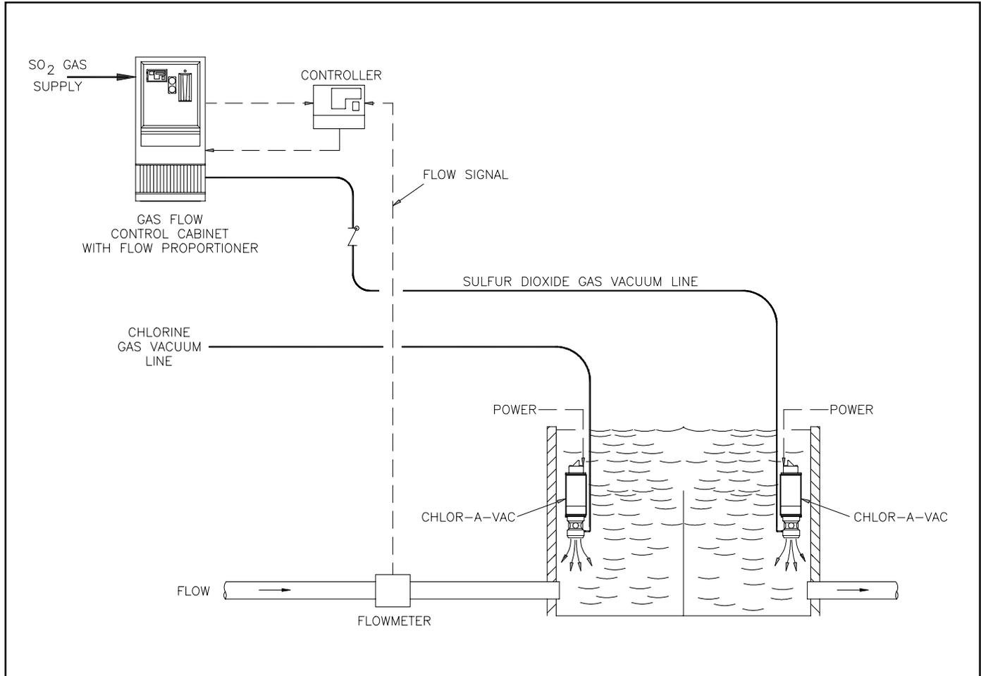
Figure 5 - Flow Proportioning System
