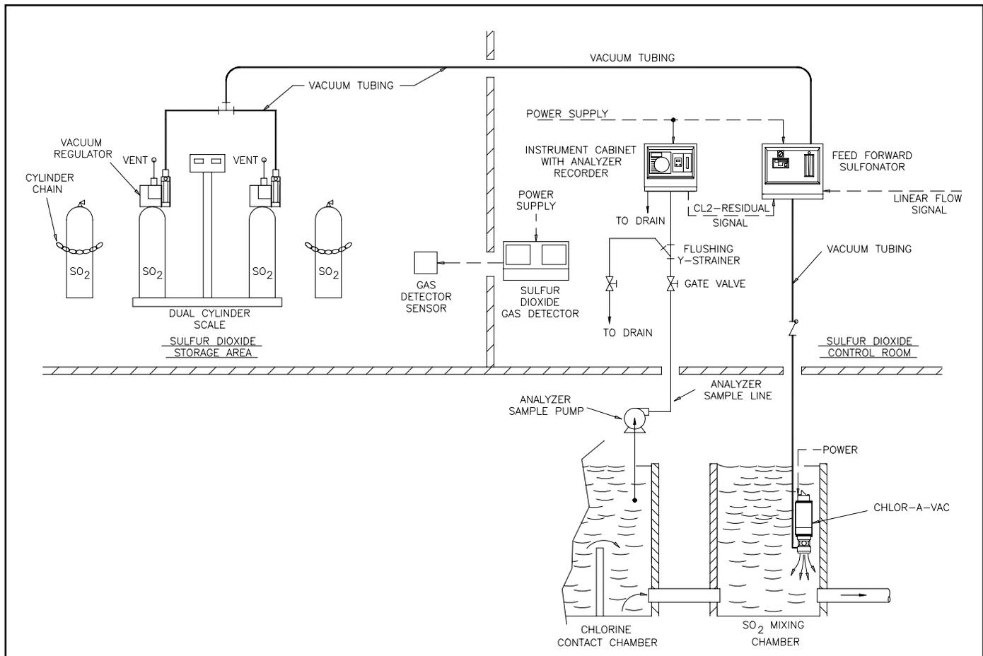
Figure 2 - Typical Cylinder Mounted Dechlorination System
