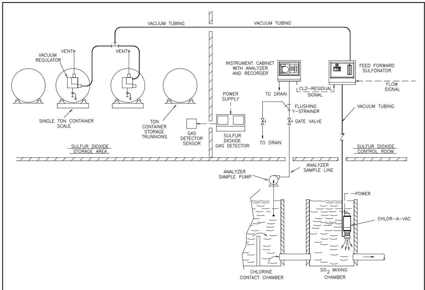
Figure 3 - Typical Ton Container Mounted Dechlorination System
