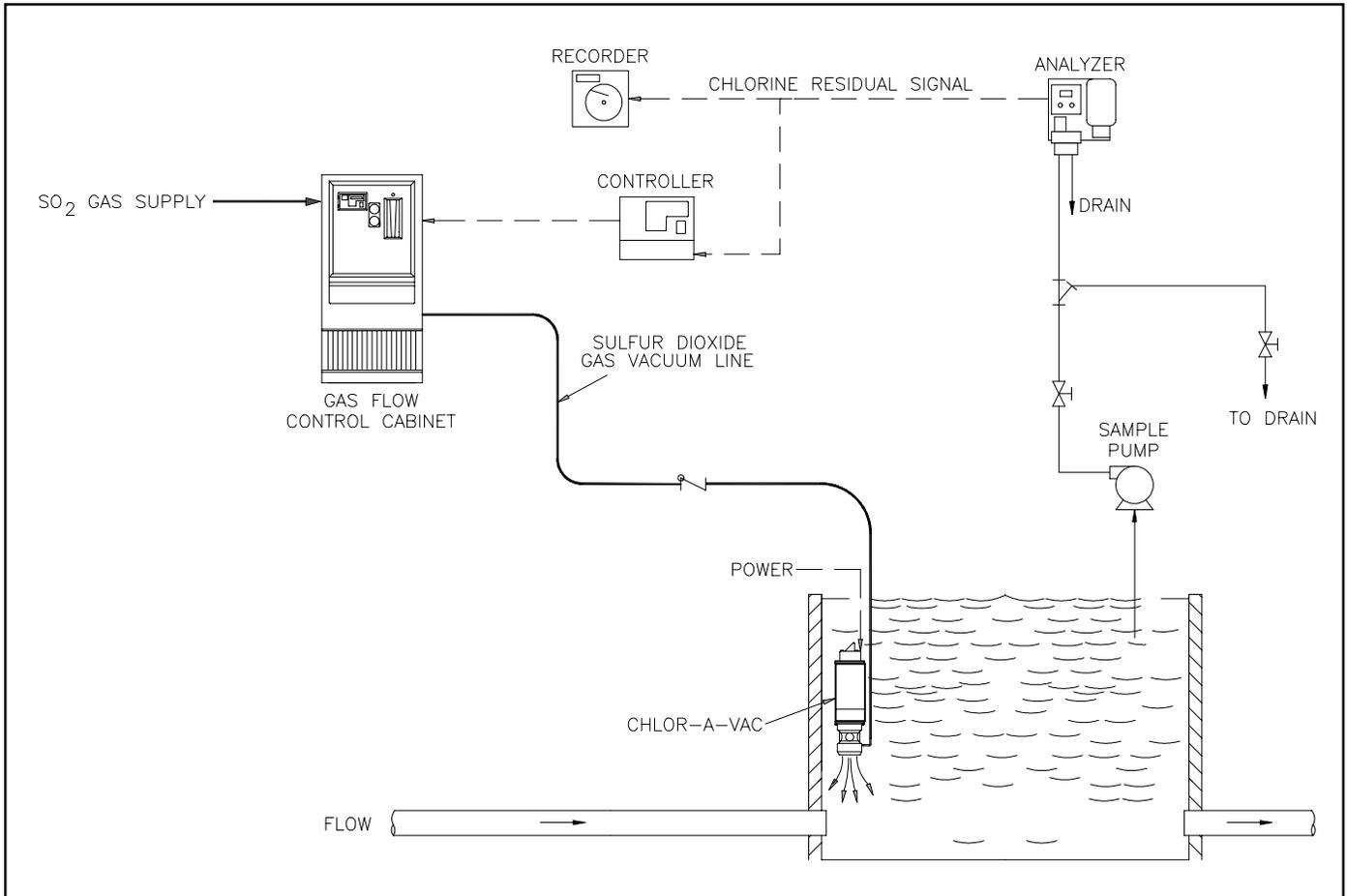
Figure 6 - Residual Control System
