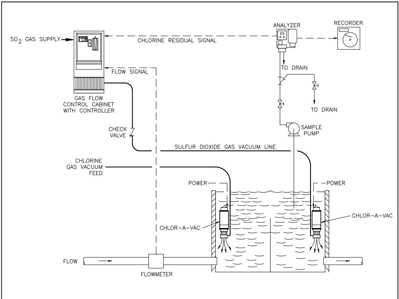
Figure 4 - Feed Forward System
